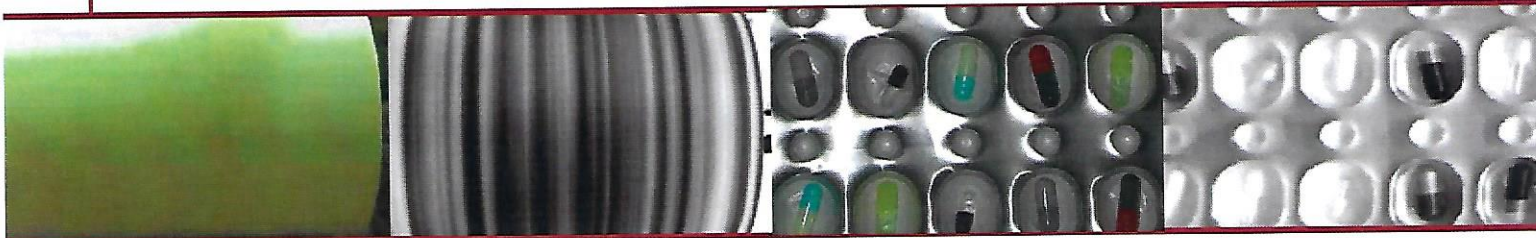
Moisture detection in paper: visible vs. SWIR
