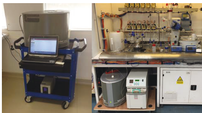
Left: photo of a mobile Spinsolve, mounted on a wheeled cart. Right: photo of a Spinsolve integrated into an automated flow chemistry system.
